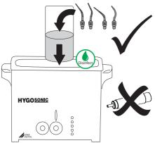
Place the handpiece without covers in a container with fluid. The drive mechanism of the handpiece must not lie in the fluid (malfunction). Therefore observe instructions concerning maximum fluid level for the Scaler handpiece.
