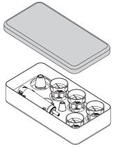
All parts which can be sterilised are optimally stored in the special Vector Scaler steri-box. For steam sterilisation the steri-boxes are placed in the small steam steriliser, "13 Reprocessing". If sterile storage is required, wrap the steri-box in suitable sterilisation packaging in accordance with DIN11607-1 and seal.
