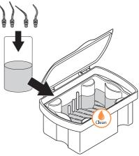
Rinse handpiece through at least 3 times using a 20-ml disposable syringe.
