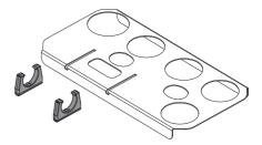
The rubber clips on the carrier plate can be replaced if necessary.
